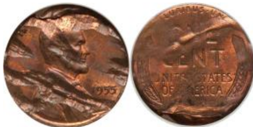
Sample of defective planchet - http://coinauctionshelp.com
