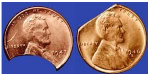
Examples of Curved and Straight Clipped Planchet error coins - https://www.fleur-de-coin.com
