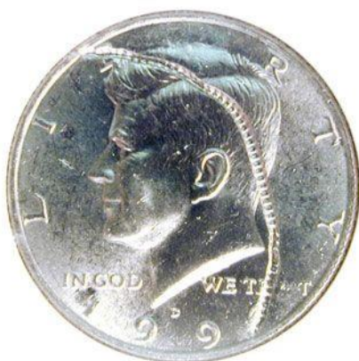
Example of strike through error 199X-D Kennedy Half-Dollar. https://www.pinterest.com/pin/526006
