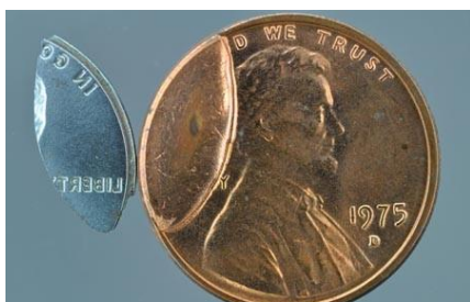
Example of a die cud error: 1975-D Cent with cud on the left where the piece of die shown broke away. https://www.ngccoin.com . Photo courtesy of Dave Camire of NCS and Andrew Steiner of Harlan J. Berk, Ltd.
