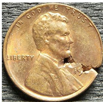
Sample of defective planchet http://www.lincolncentresource.com
