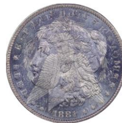
Clashed Die error on 1881-O Morgan Dollar. http://www.1881o.com/clashing.html
